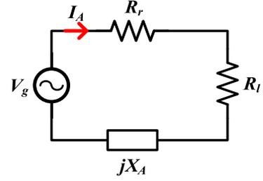
Fig. 2. Impedance model of an antenna.
