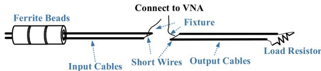
Fig. 12. Measurement setup for antenna impedance measurement.
