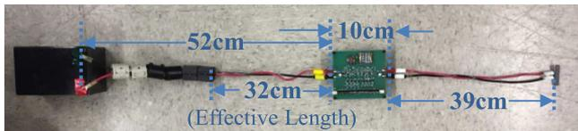
Fig. 11. Prototype of the DAB converter.
