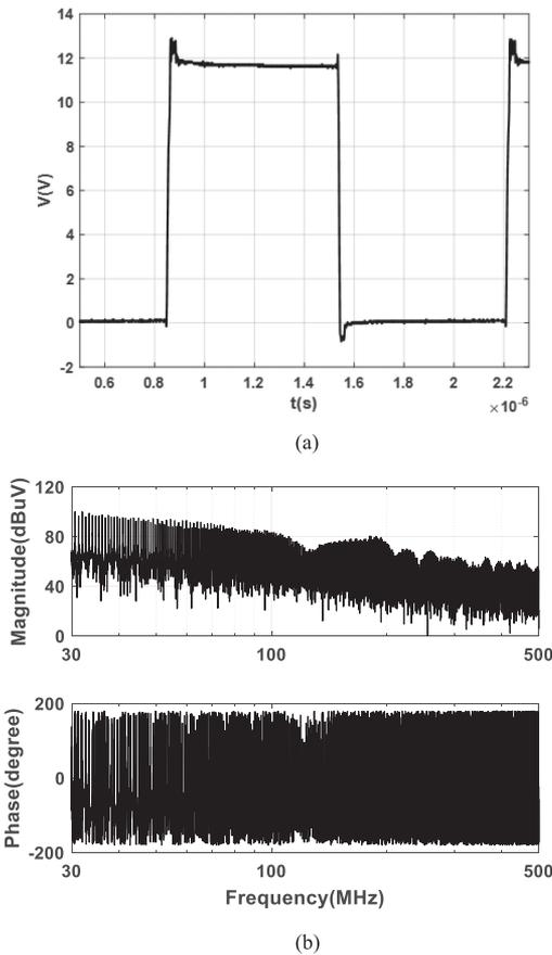
Fig. 15. Develop radiation model for  $V_{M1}$ . (a) Measured time domain waveform of  $V_{M1}$ . (b) Spectrum.
