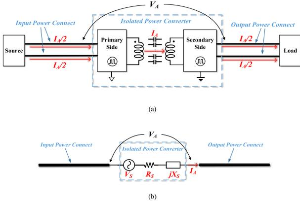
Fig. 1. Radiation mechanism of an isolated power converter. (a) CM current flowing through the parasitic capacitance between transformer windings. (b) Equivalent model.
