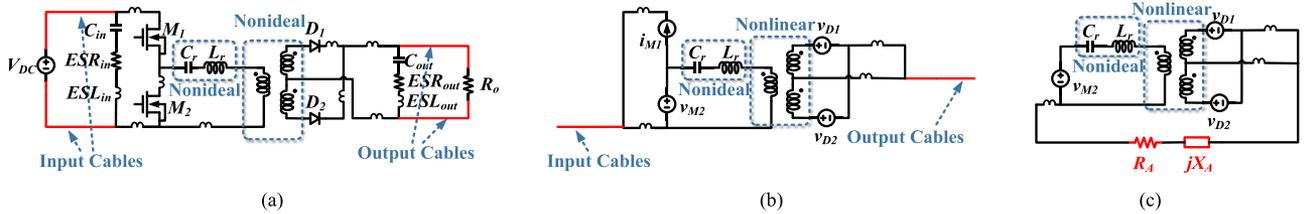
Fig. 10. Radiation model of a half-bridge LLC converter. (a) Converter circuit. (b) Substituting nonlinear devices with voltage and current sources. (c) Final radiation model.
