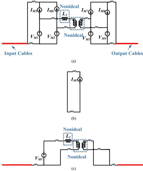
Fig. 6. (a) Radiation model for a DAB converter. (b) Noise model of  $I_{M5}$ . (c) Noise model of  $V_{M1}$ .
