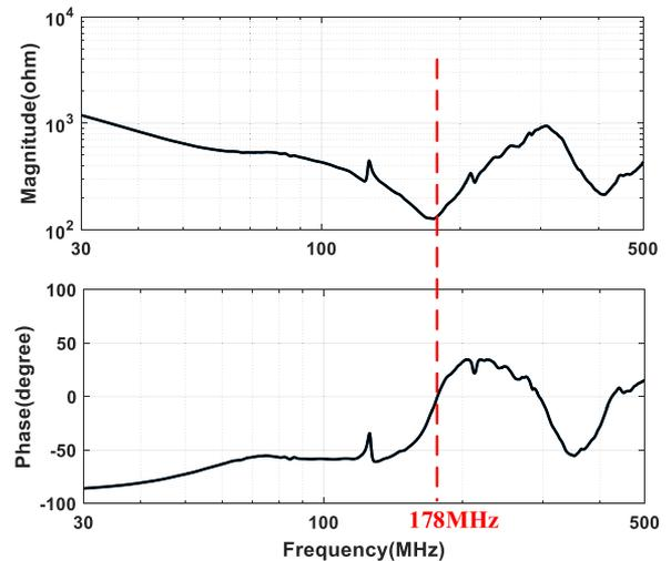
Fig. 13. Measured impedance of the antenna.
