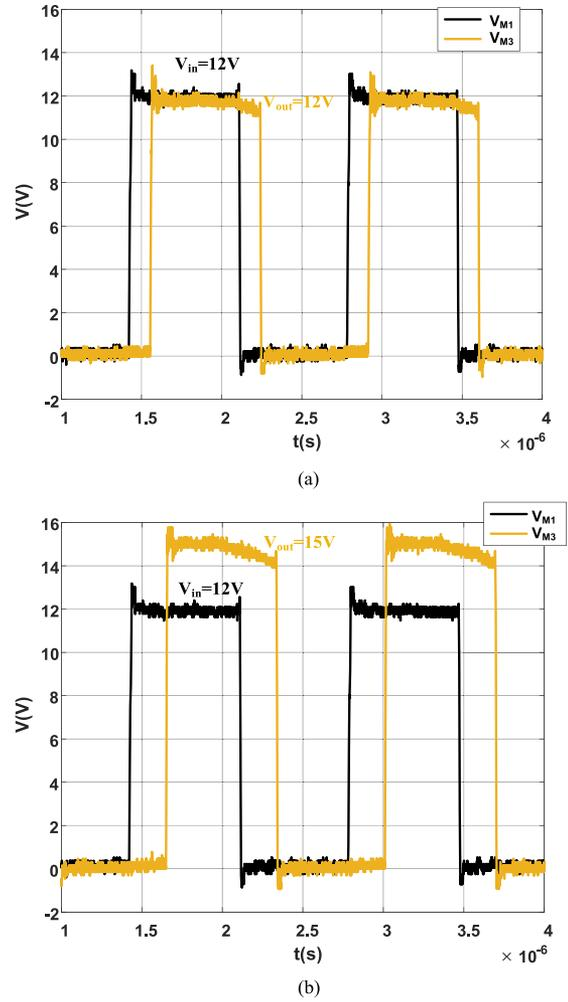
Fig. 23. Time domain waveform of  $V_{M1}$  and  $V_{M3}$ . (a) When output voltage is 12 V (7.2 W). (b) When output voltage is 15 V (11.3 W).
