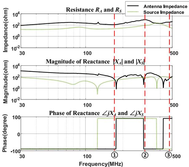
Fig. 25. Interaction of converter source impedance and cable antenna impedance.
