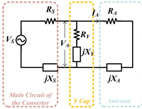
Fig. 27. Radiation model for an isolated converter with a Y-cap.
