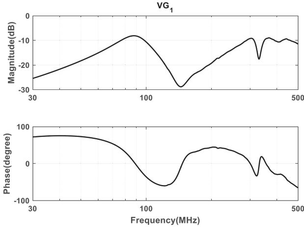
Fig. 17. Extracted  $V_{G1}$  based on the measured  $S$ -parameters.
