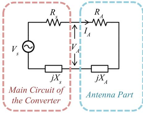
Fig. 3. General radiation model of an isolated power converter.
