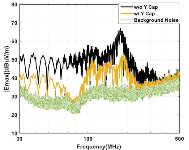
Fig. 29. Comparison of the radiated electric field  $E_{\max}$  with and without the Y-cap.
