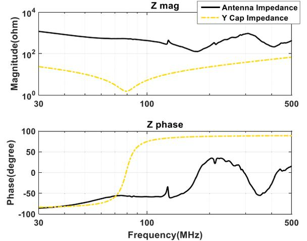
Fig. 28. Comparison of antenna's impedance and the impedance of the Y-cap.
