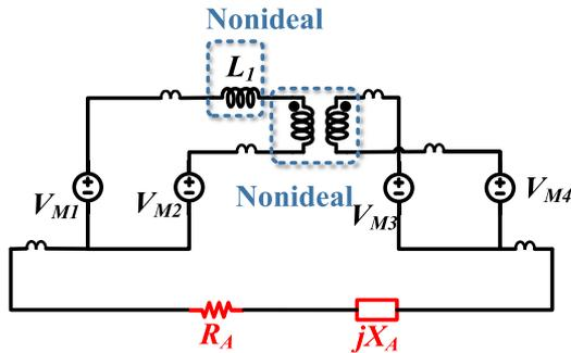
Fig. 7. Simplified radiation model for DAB converter.
