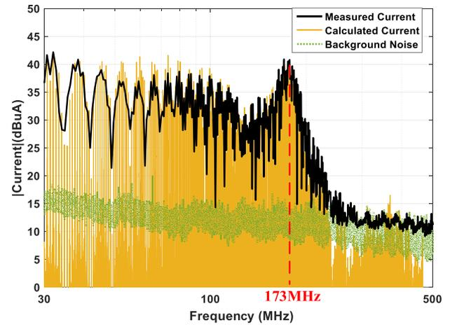
Fig. 20. Comparison of the measured and predicted CM current  $I_A$ .
