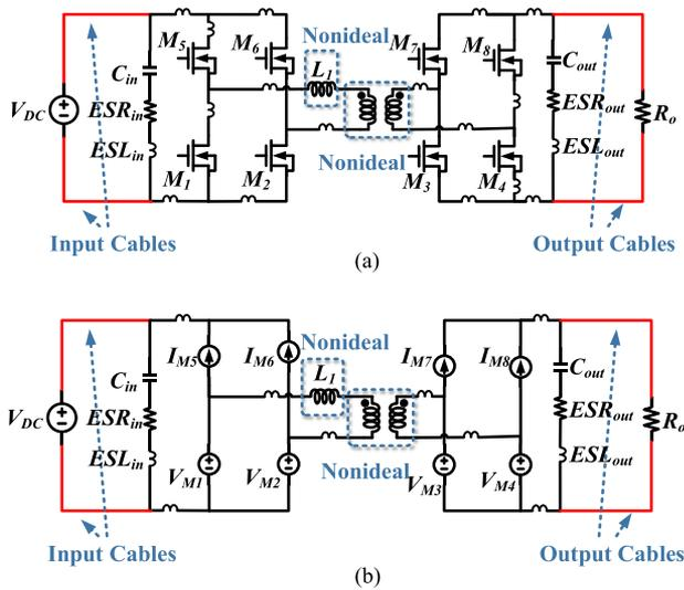
Fig. 5. DAB converter under investigation. a) Circuit. b) MOSFETs replaced with voltage and current sources based on substitution theory.
