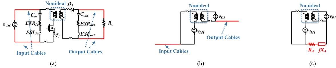
Fig. 8. Radiation model of a flyback converter. (a) Converter circuit. (b) Substituting nonlinear devices with voltage and current sources. (c) Final radiation model.
