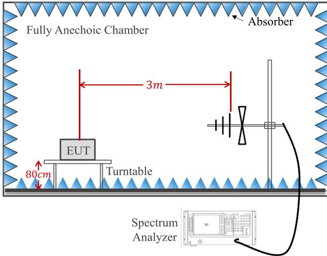
Fig. 22. Electric field measurement setup in a 3 m fully anechoic chamber.
