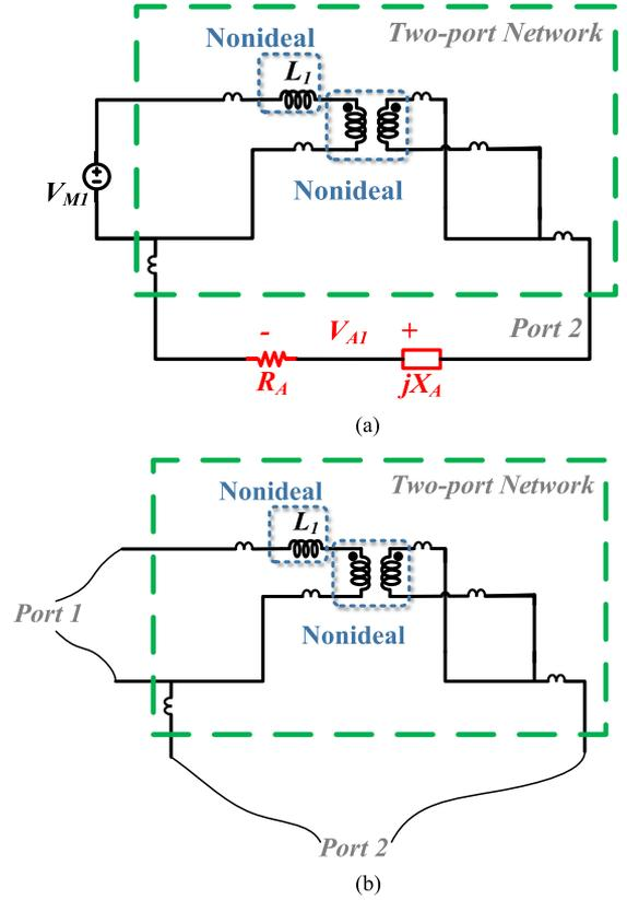
Fig. 16. Developing radiation model for  $V_{M1}$ . (a) Two port network to find voltage gain. (b) Measurement setup for  $S$ -parameters.
