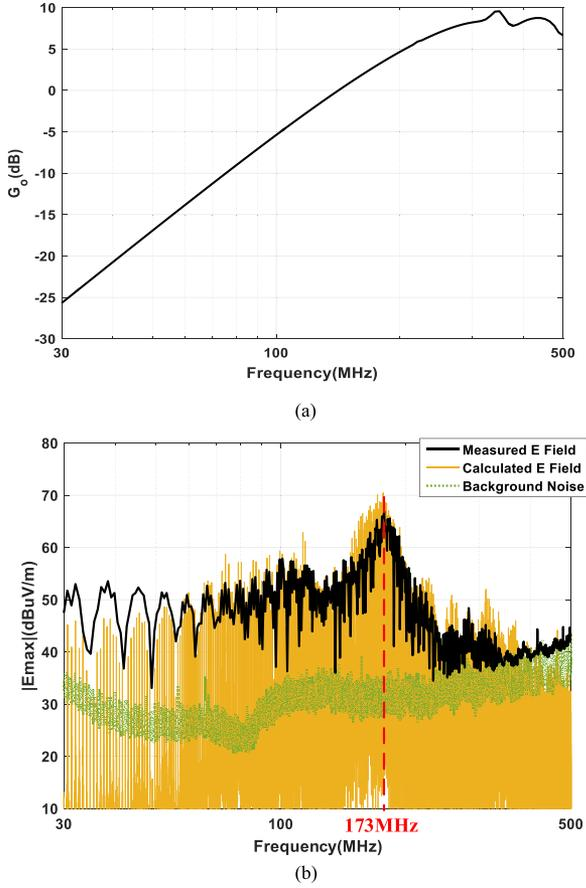
Fig. 21. (a) Simulated gain of the cable antenna. (b) Comparison of measured and calculated  $E_{\max}$ .
